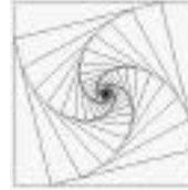
Figure 6. Iterative process of scaling and rotation two-dimensional transformations.
